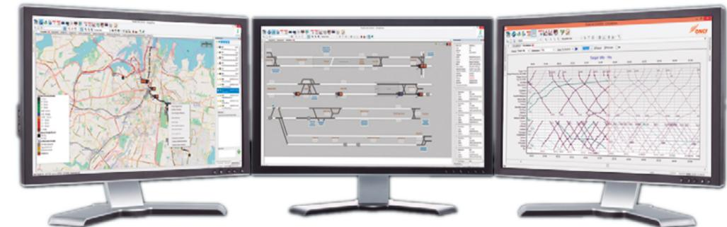
**SAE-R**®'s innovative interfaces offer different views to represent trains and stations in real-time (i.e. GIS, classic synoptic, vertical synoptic view). Every view implements specific graphical tools to manage its elements.
