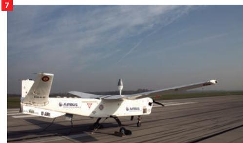
7. In October 2014 the tactical unmanned aerial vehicle (UAV) Atlante successfully makes its first flight from Deblin airbase in Poland. This is the first demonstration flight outside Spain. GMV is responsible for the flight control computer (FCC), which controls, guides and navigates the aircraft. GMV is also supplying the automatic take-off and landing (ATOL) system as a built-in part of the ground control station (GCS).
