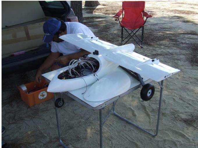
**Figure 3-2: Avionics Bay of the Flight Demonstrator**
