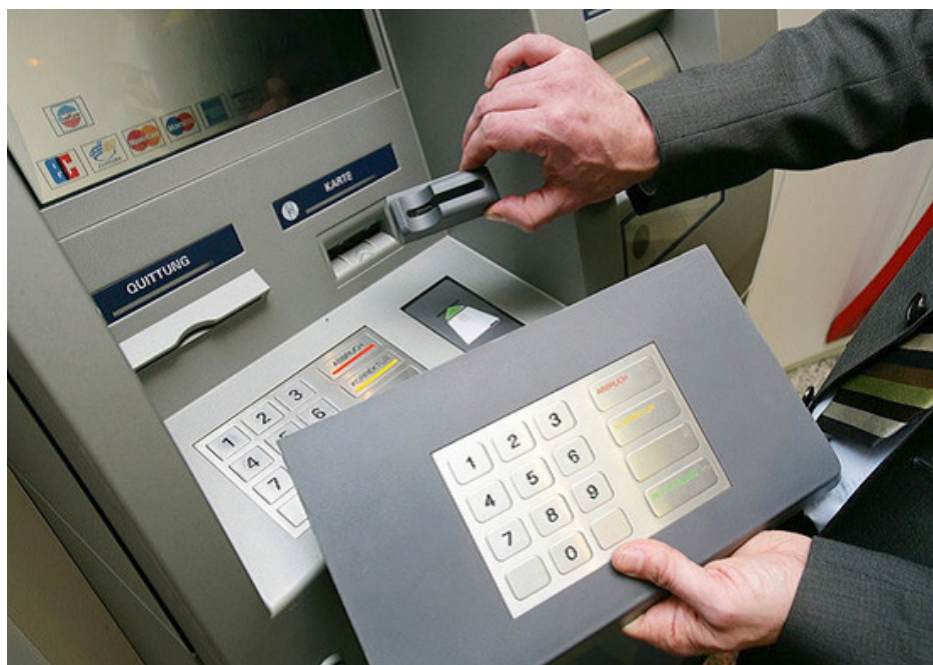
Figure 3. Old-school skimming attacks through physical means 8
