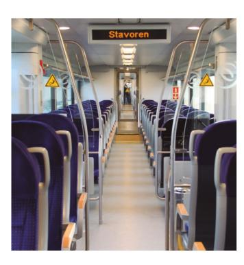
Current and next station information is shown on on-board displays and/or on-board monitors. The related audio speech is simultaneously broadcasted through the PA system of the train.
