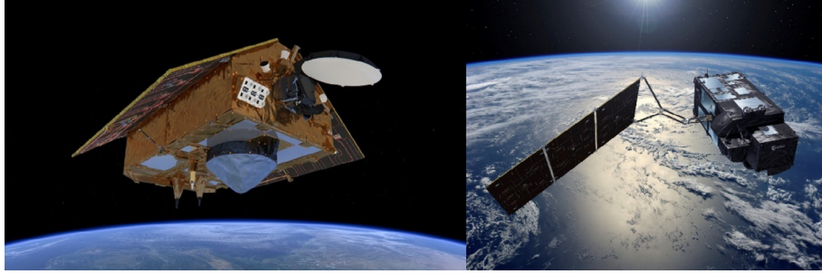
Fig. 16. Sentinel-6 (left) (credit: ESA/ATG medialab) and Sentinel-3 (right) (credit: ESA-Pierre Carril). The roof of Sentinel-6A together with the large \beta -angle variations caused periodic shadowing of the nadir part of the satellite body. Sentinel-3 instead, does not suffer these periodic shadowing.
